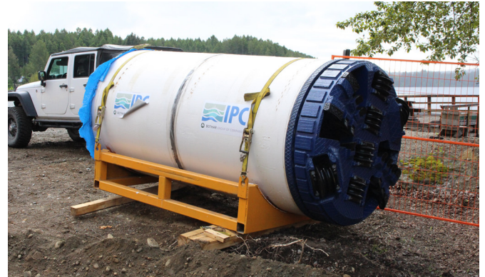
Tunnelling equipment has arrived at the pump station site. This is the microtunnel boring machine that will create a tunnel into the lake for the intake pipe.
